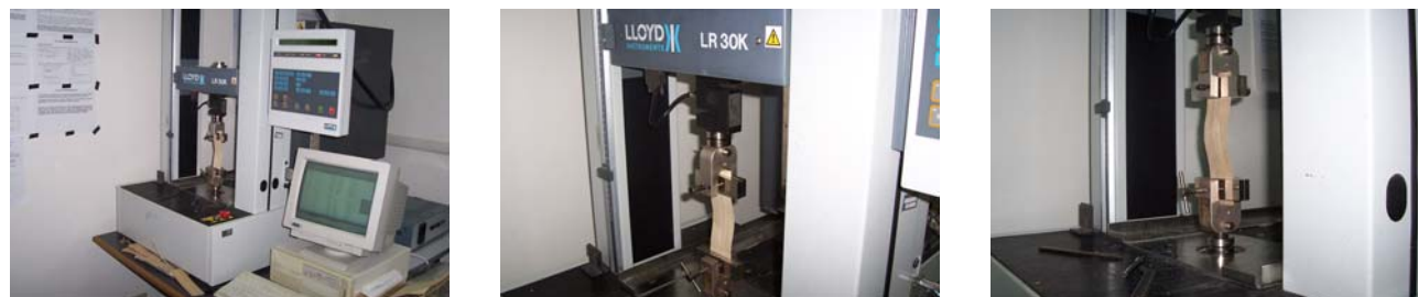
Fig. 2: Experimental tensile tests on raw bamboo unidirectional
