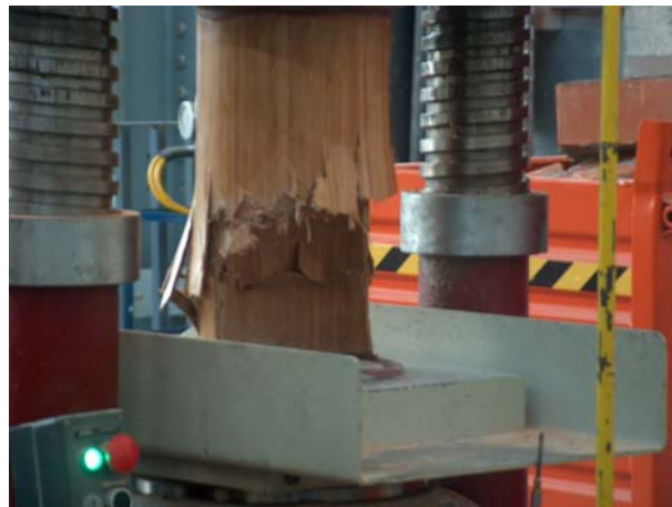
Fig. 13: Compression test on a spinnaker pole section
