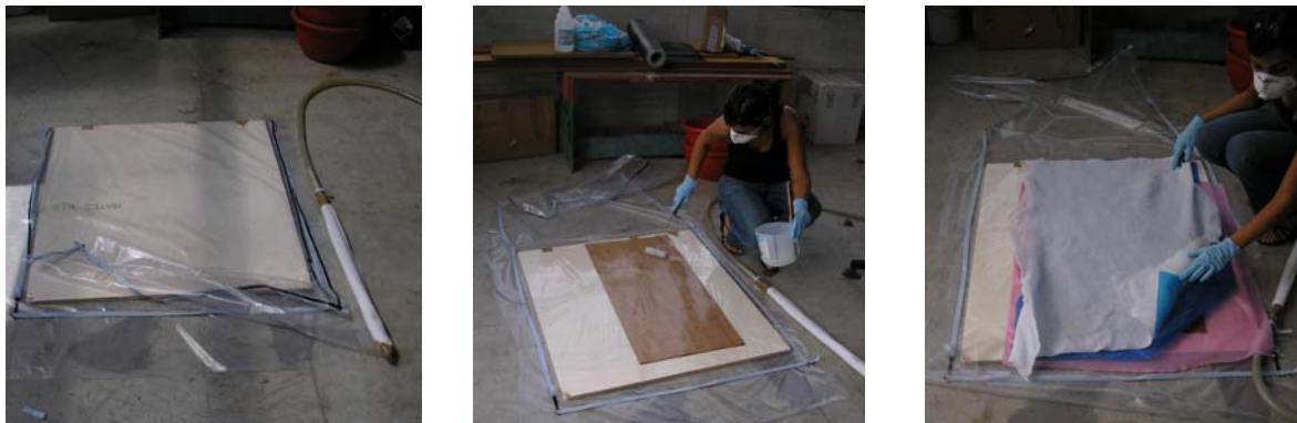
Fig. 6: Vacuum bag process for composite bamboo panels
