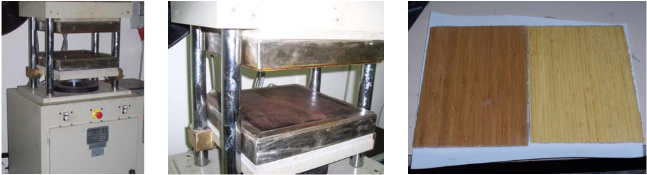
Fig. 7: Hot pressing process for composite bamboo panels
