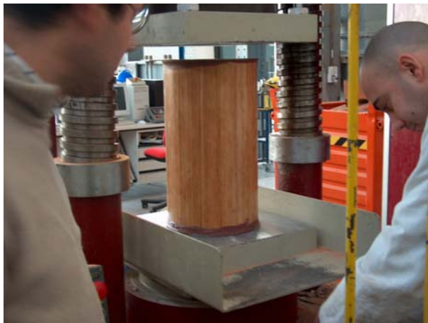
Fig. 13: Compression test on a spinnaker pole section
