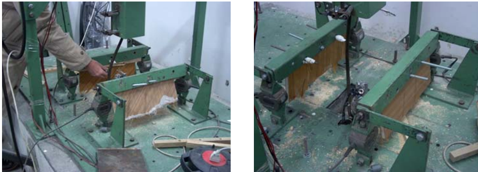
Fig. 15: Impact test on a sandwich panel.
