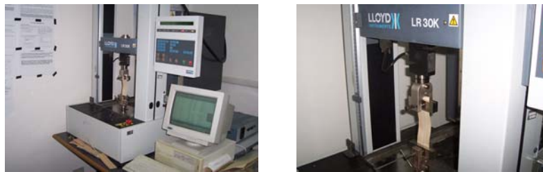
Fig. 2: Experimental tensile tests on raw bamboo unidirectional
