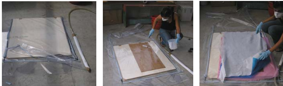
Fig. 6: Vacuum bag process for composite bamboo panels
