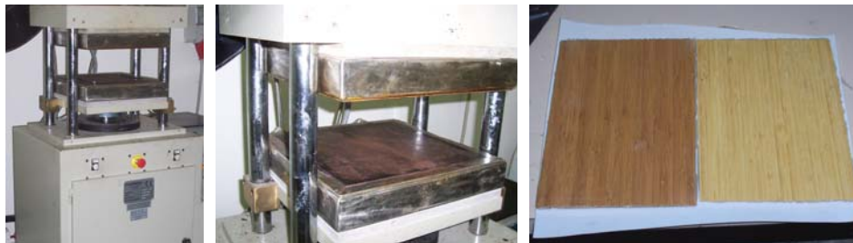
Fig. 7: Hot pressing process for composite bamboo panels
