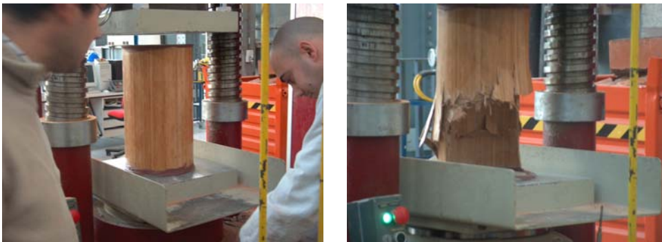
Fig. 14: Compression test on a spinnaker pole section
